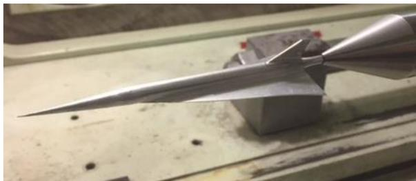
Fig. 1 HyCruise (waverider wing configuration)
