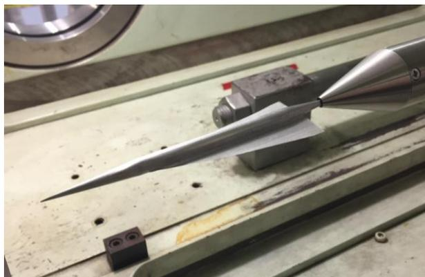
Fig. 1 HyCruise (waverider wing configuration)
