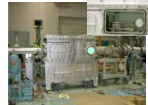
Hypersonic wind tunnel measurement section: airflow from right to left, the centre circle is the observation window and the nozzle section is visible on the right).
