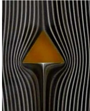
**Figure 13** Flow pattern around a triangular plate with vertex up.
