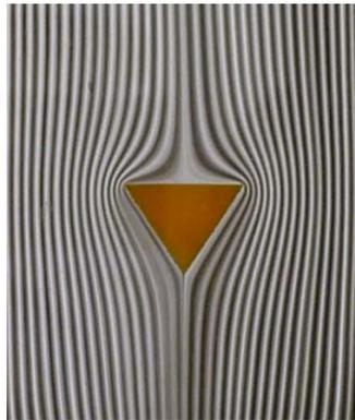
**Figure 14** Flow pattern around a triangular plate with vertex down.
