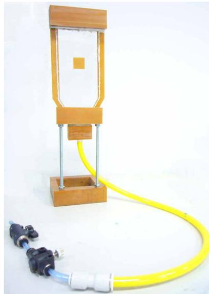
**Figure 9** A view of complete Hele-Shaw device assembly.
