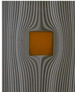
Figure 12 Flow pattern around a square plate.
